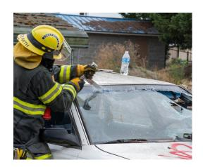
The Extrication Tomahawk also removes plastic trim, valves stems, rubber gaskets, and is great for cutting laminated glass. This 10 tools in 1 is a must have for any auto extrication technician.
