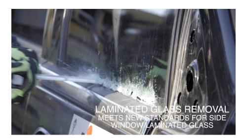
The new federal motor vehicle safety standard no. 226 "Ejection Mitigation" is designed to reduce the partial and complete ejection of vehicle occupants through side windows in crashes, particularly rollover crashes, by using "laminated glass" in all side windows in 2018.
