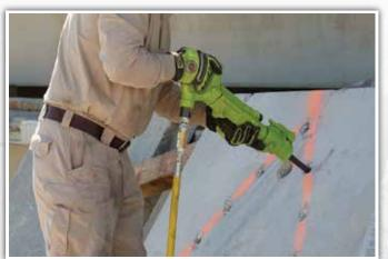
that allows the rescue technician the ability to quickly and easily change bits. In addition, each tool has been specifically designed to enable one operator to use and control each tool. This allows other technicians to be deployed to other critical operations.
